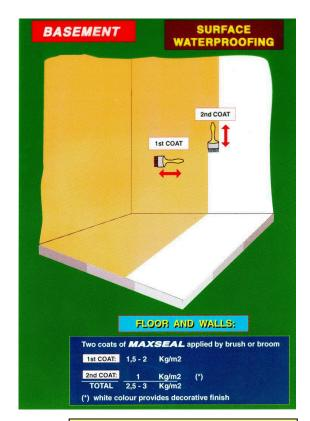
Two coats of MAXSEALFLEX applied by brush or broom
