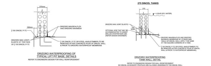
BASEMENT CONSTRUCTION AND DRIZORO WATERPROOFING FOR PERMANENT WATER TABLE ABOVE THE FOOTING LEVEL
